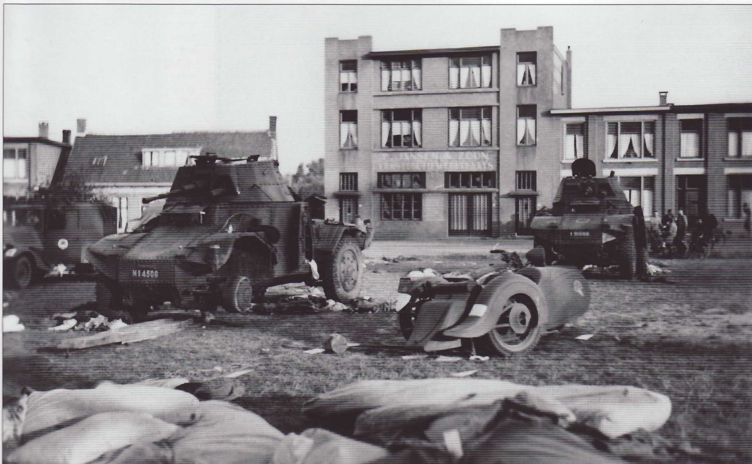
Two photographs showing knocked out enemy vehicles inside a French town captured by one of the "Das Reich" units. The photos show the famous "Panhard" armored car, which was one of the very best such vehicles in the world at this time. This 4x4 armored car was designed for the French Army before the war. It had a crew of four and was equipped with a 25mm main armament and a 7.5mm coaxial machine gun.
