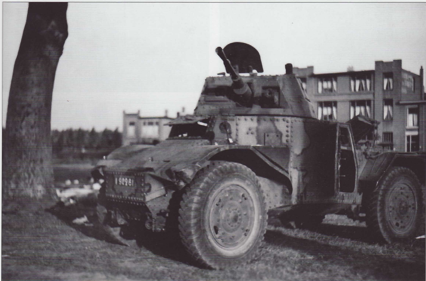
Two photographs showing knocked out enemy vehicles inside a French town captured by one of the "Das Reich" units. The photos show the famous "Panhard" armored car, which was one of the very best such vehicles in the world at this time. This 4x4 armored car was designed for the French Army before the war. It had a crew of four and was equipped with a 25mm main armament and a 7.5mm coaxial machine gun.
