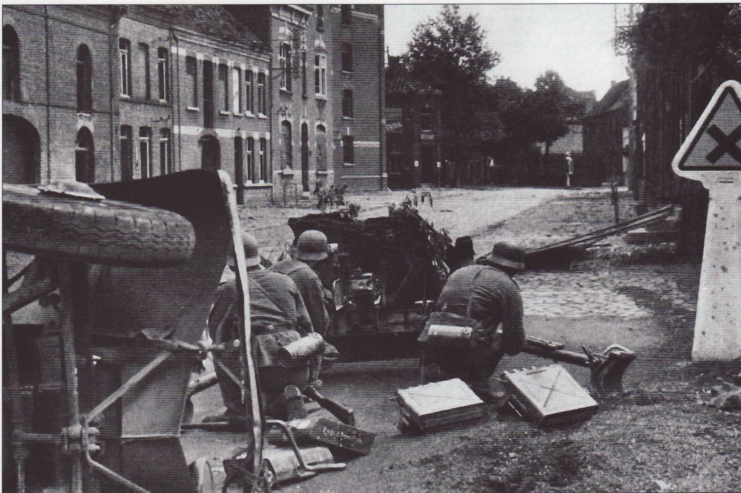
A PaK35/36 crew guards the approaches of road in a town in northern France. The PaK35/36 became the standard anti-tank weapon in both the Wehrmacht and Waffen-SS during the early part of the war. It weighed only 432kg and had a sloping splinter shield that afforded minimal protection for the crew. (RM collection)
